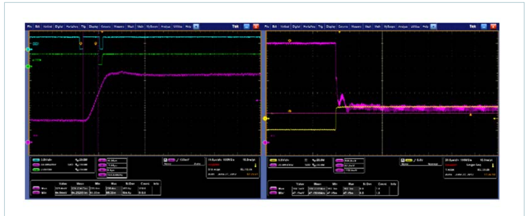
Figure 12 Response to a 1.05 – 1.2V set point transient at 108A load (left) and a 34 – 165A load transient (right)
